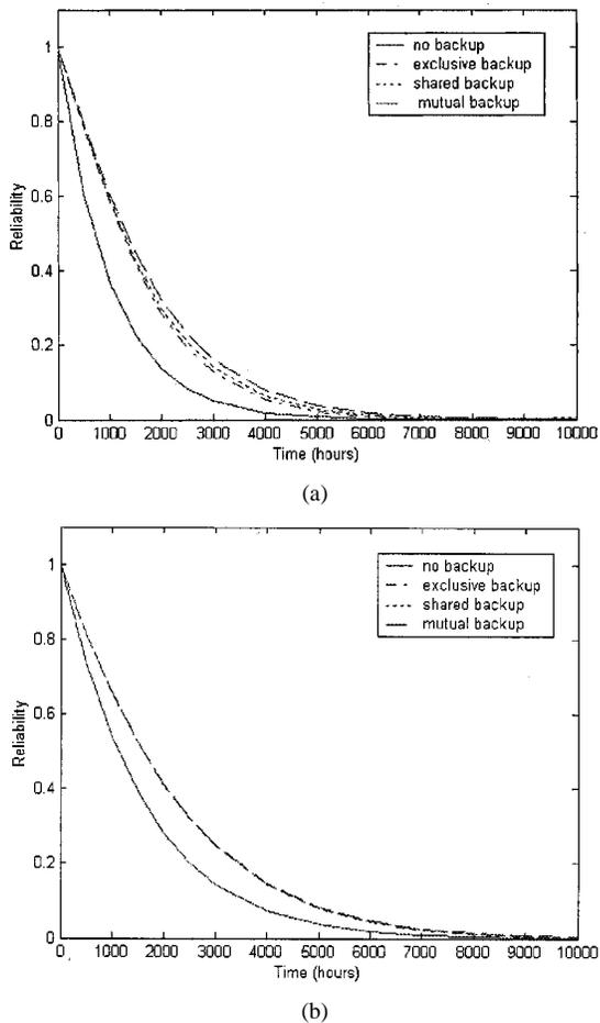
Fig. 5. (a) System reliability without repair. 1 Server and 1 Bus in both control center and substation. Failure rate of components:  $1E-5$ . (b) System reliability without repair. (1+1) Server in both control center and substation. Failure rate of components:  $1E-5$ .
