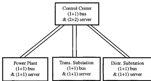
Fig. 2. Full redundancy configuration of operation and control system.
